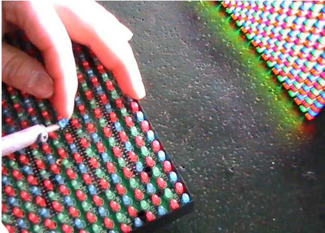
Using the searing-iron to remove the bad lamp (picture 2)
